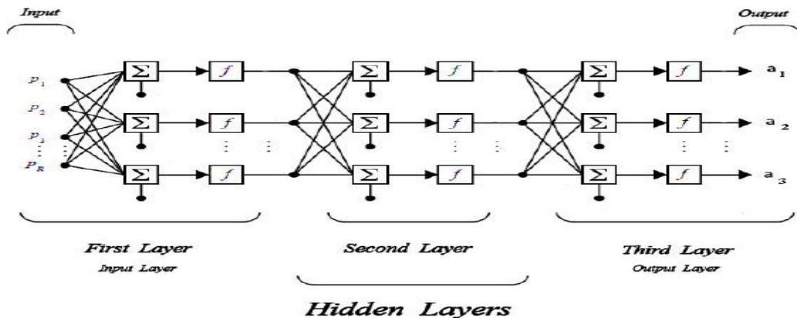
Figure 1. A schematic of ANN and its layers
